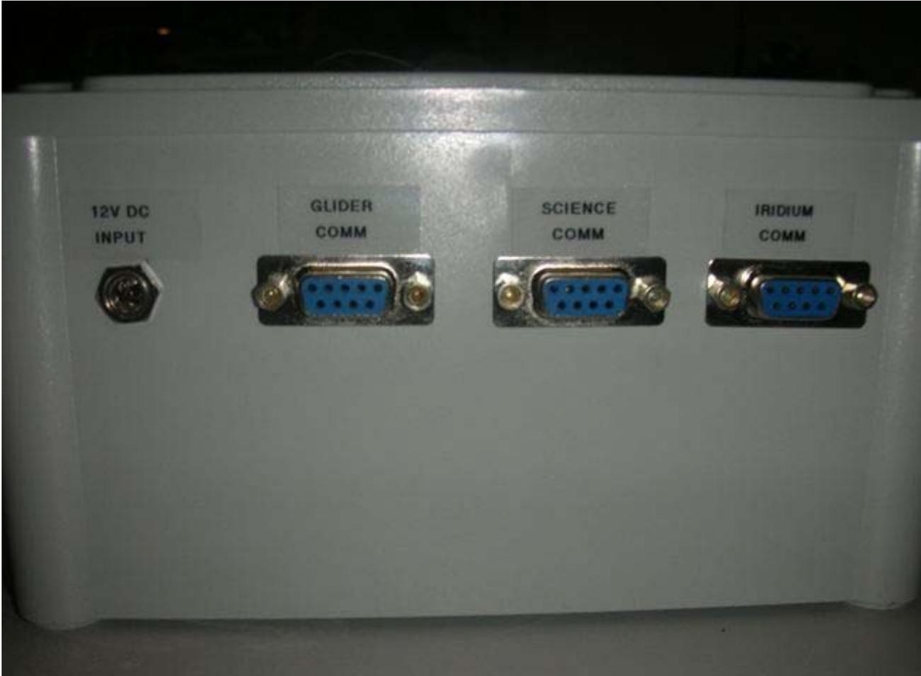
From left to right: External power 12 VDC, glider freewave connection, direct science connection, Iridium modem connection
