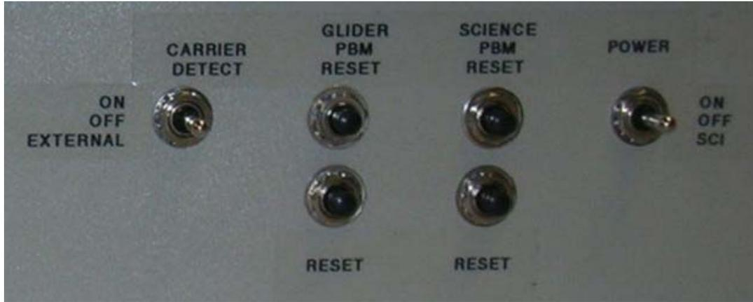
**From left to right: Carrier detect selection, glider persistor reset, science persistor reset, power on/off/science selection**
