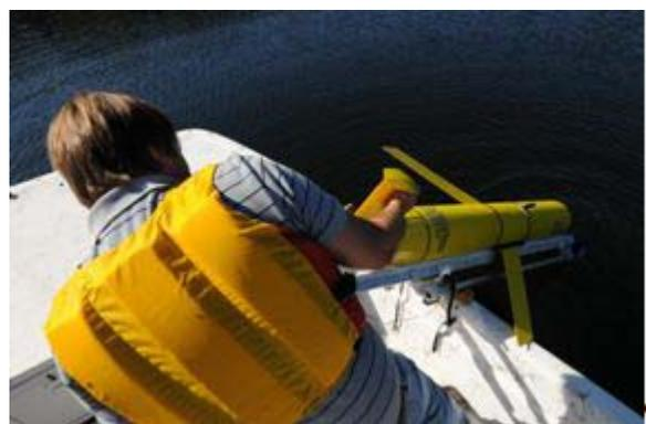
Lower the cart with nose ring into water, and manipulate the glider by the tail boom into position on the cart. Lift and tilt the glider onto the ship's deck.
